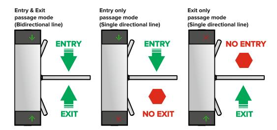
The system calculates each entry or exit pass through turnstiles. When the number of visitors inside of the controlled area is more than the permissible number, all entrances will be blocked and all exits will remain open.
