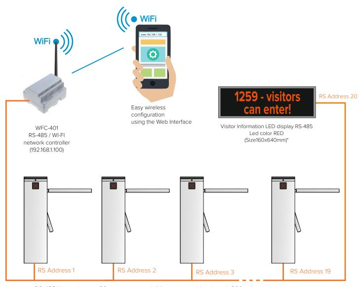
RS-485 Network up to 20 units in network (Maximum total line length 200m \*)
